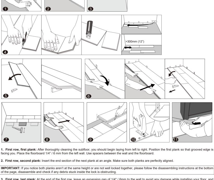
3. First row, last plank: At the end of the first row, leave an expansion gap of 1/4" / 6mm to the wall to avoid any damage while installing your floor, and measure the length of the last plank to fit.
