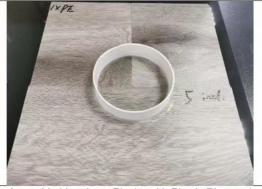
Assembled Laminate Planks with Plastic Ring seal
